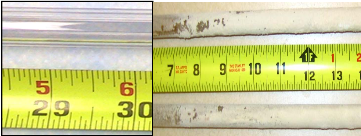
Figure C-13. Comparison of (left) clean quartz rod and (right) dirty quartz rod exposed to flue gas downstream of ESP at MRY Unit 1 for sixteen days.
