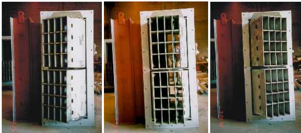
Figure 2 - TLN Separated Overfire Air Windbox with Horizontal Yaw and Vertical Tilt Control
