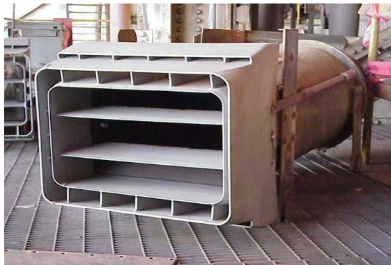
Figure 4 - Foster Wheeler's Double Shroud Coal Nozzle Tip
