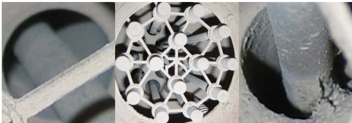
Figure C-17. Images of top of DBD reactor showing ash accumulations on electrodes and reactor surfaces.
