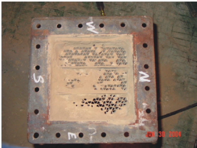
Figure 31. Pictures of catalyst inlet after about 4 months of exposure to flue gas and particulate.
