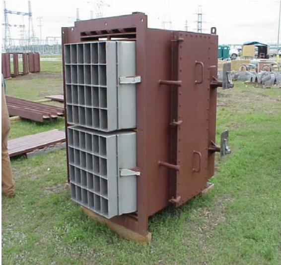
Foster Wheeler SOFA Windbox with two “double shroud” nozzle tips
