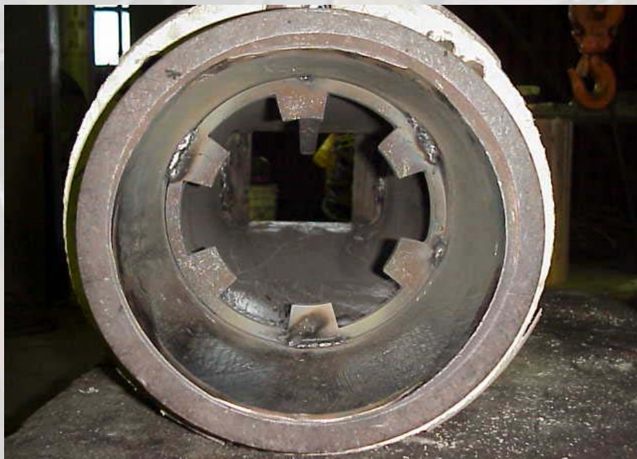
ACT Rope Breaker positioned inside existing coal pipe
