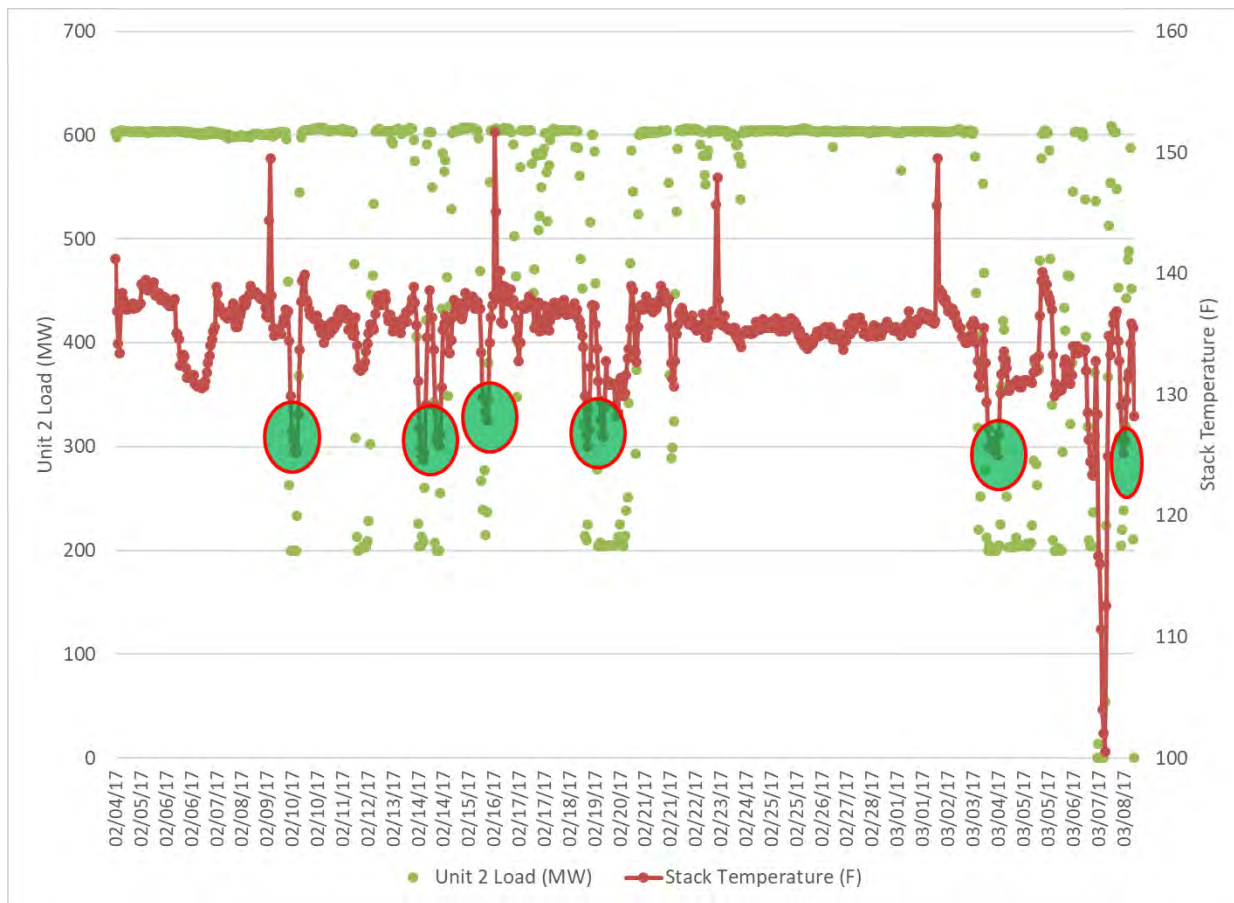
Figure 2-6: Winter 2017 Test Case Results of Unit 2 Load v. Stack Temperature
