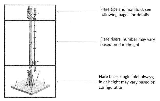
Note: The figures in Appendix A show various multi-tip configurations with the model SHC-6 tip. These configurations can also utilize model SHP-6.
