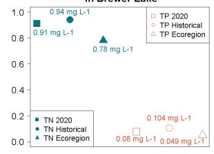
**Figure 4.** Median concentrations of TN and TP in mg L<sup>-1</sup> compared to regional medians
