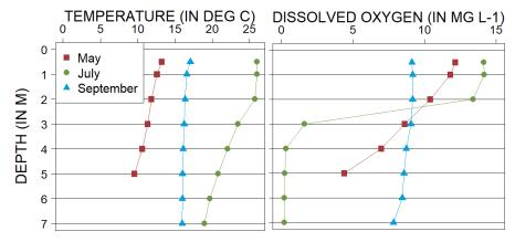
Figure 2. 2016 profiles of temperature (left) and dissolved oxygen (right) in milligrams per liter (mg L<sup>-1</sup>)
