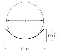
TANK/SADDLE ELEVATION DETAIL
