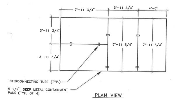
EXCESS CONTAINMENT CAPACITY = CONTAINMENT CAPACITY - VOLUME OF LARGEST CONTAINER
