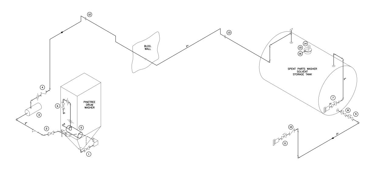
SPENT PARTS WASHER SOLVENT PIPING SCHEMATIC
