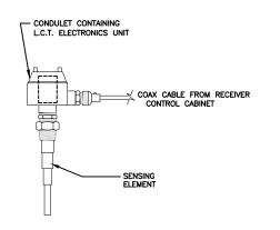
L.C.T. SENSING ELEMENT AND CONDULET DETAIL
