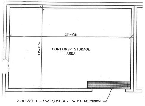
CONTAINER STORAGE AREA WITH CONCRETE SLAB AND CONCRETE CURB AT PERIMETER. TRENCH AT DOOR OPENING.
